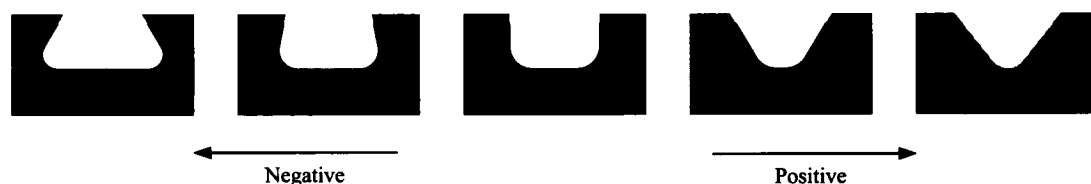
Figure 1. Various etching profiles from a DRIE process.
